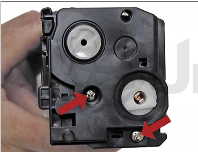
27. Install the outer gear side and cap and two screws.
